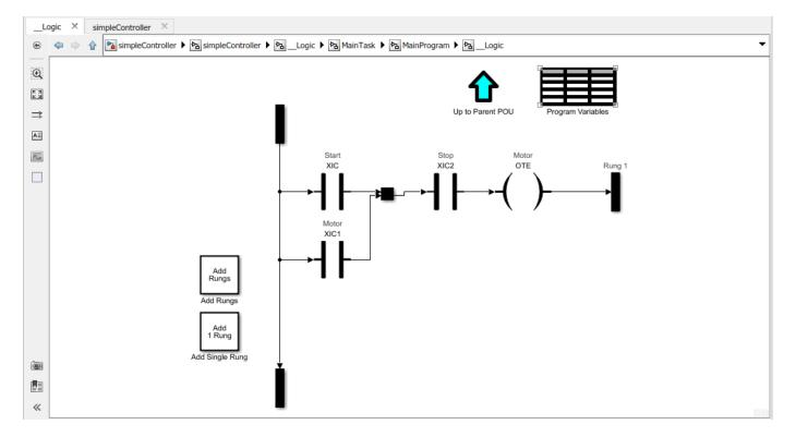
Generate code for the subsystem, simpleController/simpleController.
